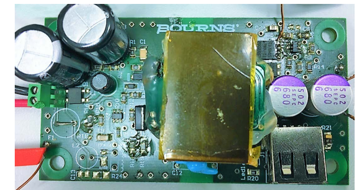
Figure 4 View of an AC/DC Adaptor with a Planar Transformer and other Bourns® Components
