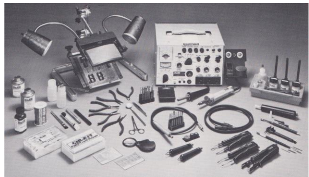
Fig. 1. PACE PRC-350 Bench Top Repair Center was an early Miniature/Microminiature electronic repair system adopted by NAVAIR's Avionics Module Repair Improvement Program (AMRIP)
