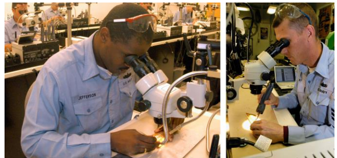
Fig. 2. During the Miniature Electronic Repair Class, students can expect to work extensively under 20x microscopes.
