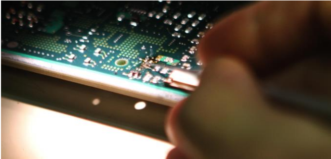
Fig. 3. A Marine Corp 2M Microminiature Repair technician in Afghanistan performs an intricate multilayer excavation. The technical skill required to successfully accomplish this task can only be obtained through 2M training.
